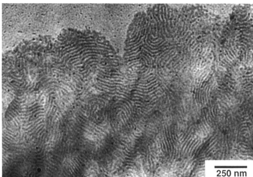
FIGURE 9 Transmission electron micrograph of 28 wt% polystyrene sample stained with ruthenium tetroxide.
